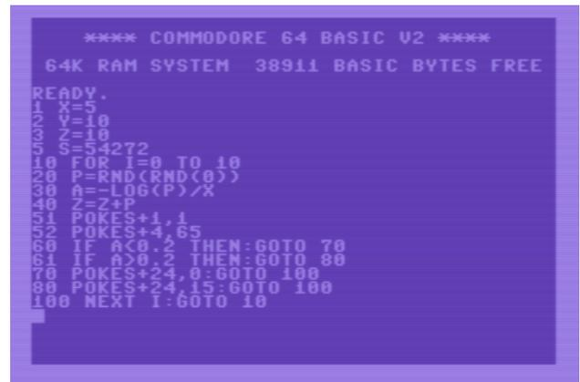
**Figure 4.** BASIC example of accessing SID addresses, assigning values, writing conditionals, and looping.
